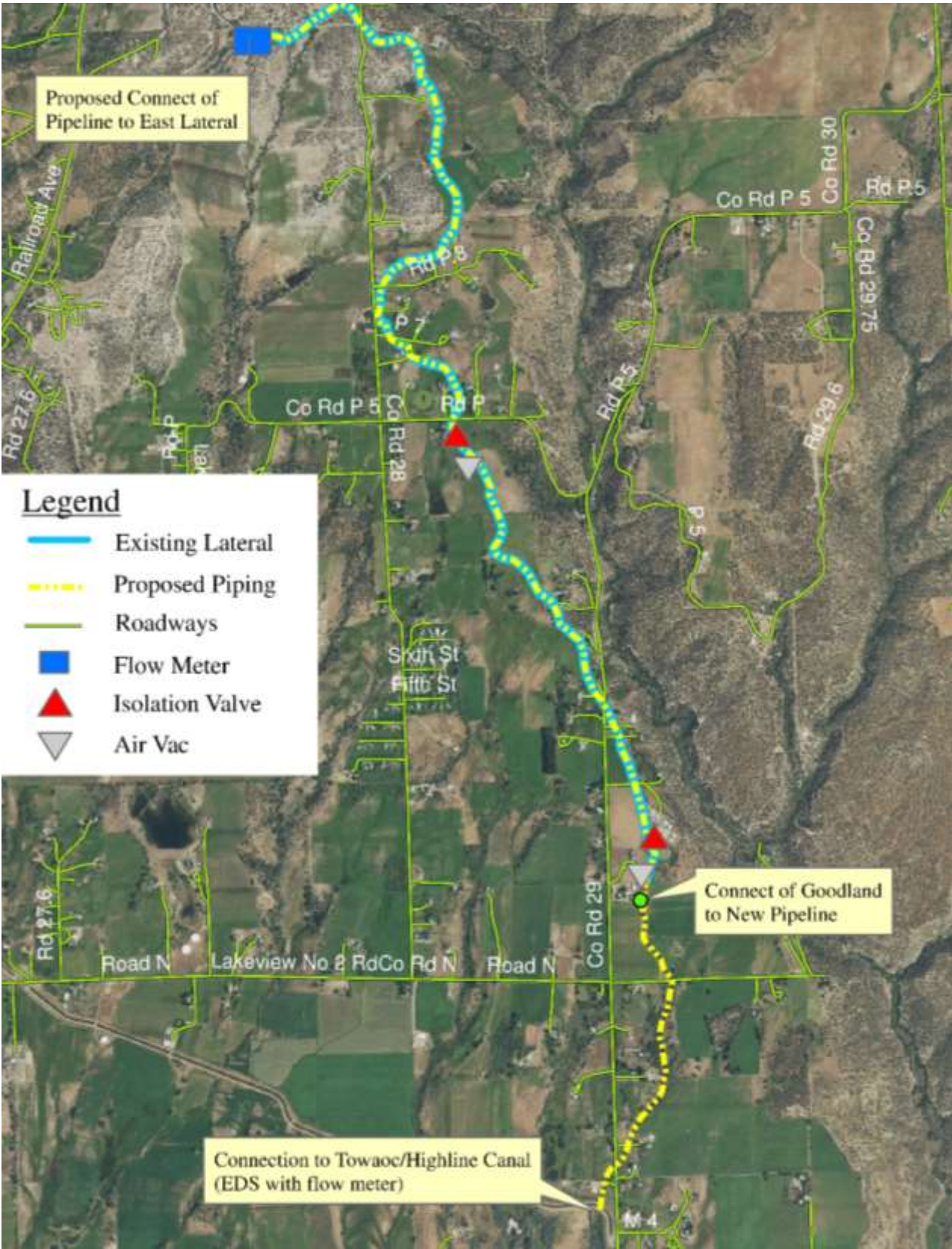
Figure 12. Goodland General Location of Pipeline Improvements
